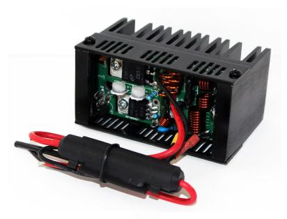
**FAN-READY FINS** The new heatsink on the RFX85 & RFX85HD is designed for mounting single and dual 40mm fans without any extra hardware
